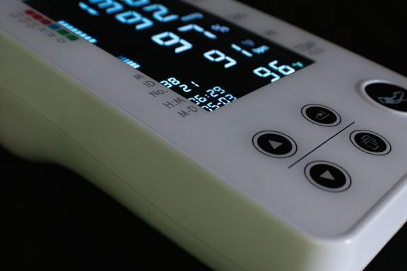
This monitor is a hand-held device that digitally captures a wide range of vitals including: temperature, blood pressure, heart rate, and pulse oximetry. The main console weighs less than 1.25 lbs and fits easily in the palm of your hand. This design combines accurate measurements of key vitals with intuitive functionality.
